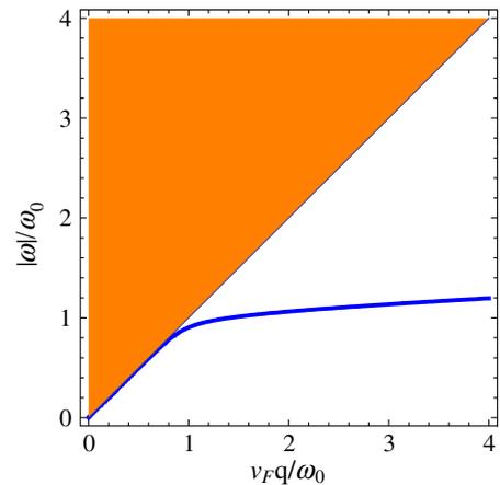
FIG. 1 (color online). Plot of the region corresponding to the  $e$ - $h$  continuum (shaded area) and the dispersion of the hybrid states made of an optical phonon and an  $e$ - $h$  pair, obtained from the poles of  $D_+$  and  $D_-$  for  $g/v_F = 1$ .
