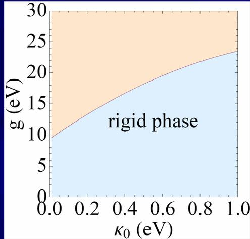
We can therefore characterize a rigid phase of graphene where it exists as a flat membrane over long-distance scales.
