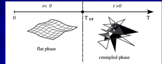
$$F = \underbrace{\frac{1}{2} \kappa \int d^D x (\partial^2 h)^2}_{\text{bending}} + \underbrace{\frac{1}{2} \int d^D x (2\mu u_{ij} u_{ij} + \lambda u_{ii} u_{jj})}_{\text{stretching}} + \underbrace{\frac{1}{2} t \int d^D x u_{ii}}_{\text{tension}}$$
