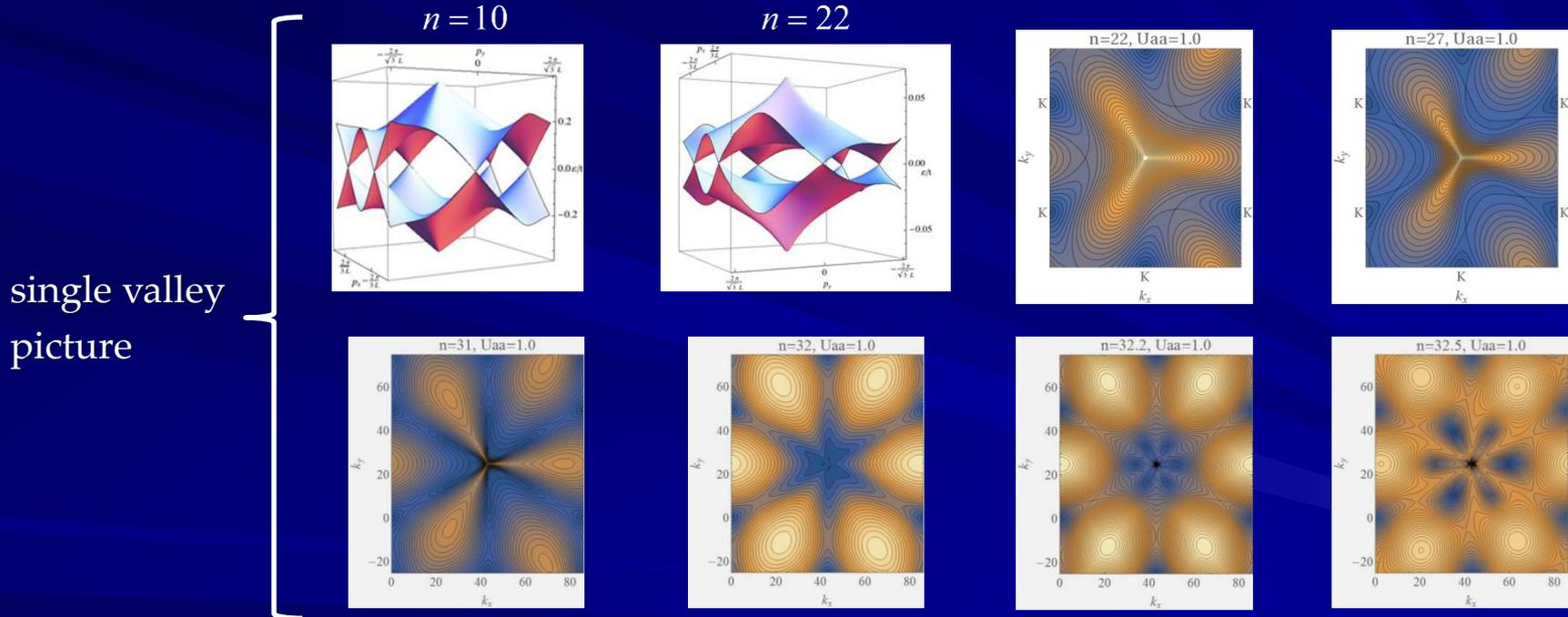
The bands are never flat, but there is a critical value of the interlayer coupling strength at which the symmetry is enlarged from  $C_{3v}$  to  $C_{6v}$ , which causes the effective compression of the bandwidth of valence and conduction bands.
